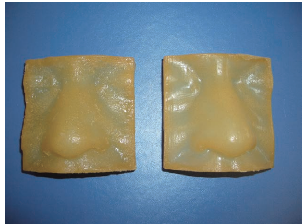
Fig. 1. Elastic model of the face with 2 layers. The surface layer is made of polyurethane with a thickness of 1 mm and the inner layer is silicone. The left model was made from computed tomographic stereolithographic data and the right from stereolithographic data from a 3-dimensional camera.
